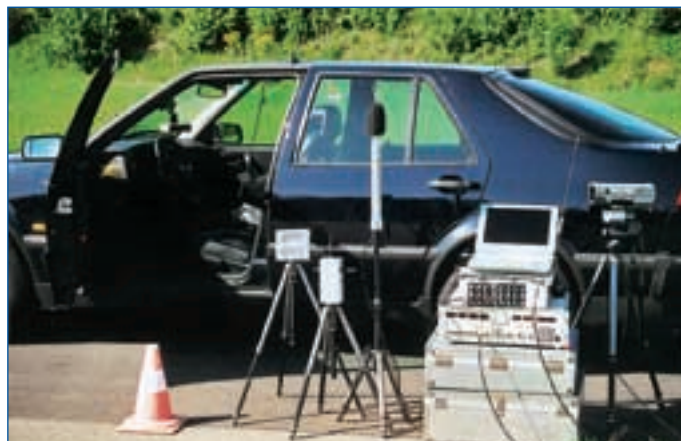
Mobile system for pass-by measurements
