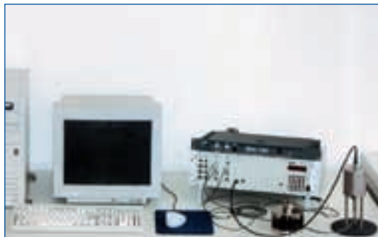
Computer-controlled transducer test system
